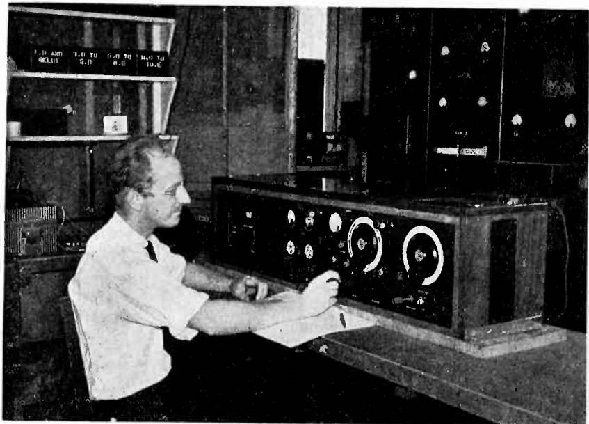
Portable frequency standard for F.C.C. being tested by J. O. Booth of Westinghouse, accurate within 3 parts in one million
