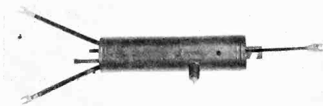
Fig. 4—Shield-grid Thyatron (3-element gas rectifier)
